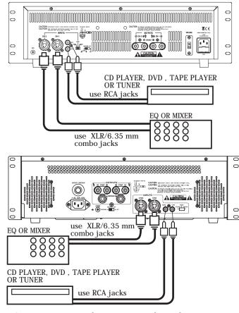
Connecting an equalizer or external signal processor Connect the processor's OUT to the amplifier's IN connector.
